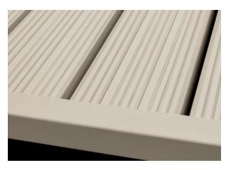
ASTRODOCK 2x6S is a good fit for any deck or marine dock application. Our unique deck board profile allows screws and fasteners to be secured within the board, then covered with snap-in inserts for a clean appearance. Made from a highly weatherable, outdoor grade PVC, this decking will provide a low maintenance surface for your dock or deck. Choose between beige and gray, both of which will remain barefoot comfortable even in direct sun light.
